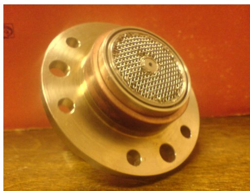
Fig. 3 Photography the one-injector mixing head of the engine DMT MAI-200-HTHP with catalyst ignition system
