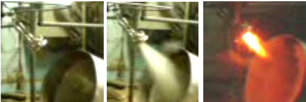
Fig. 6. Ignition test of mixing head of engine DMT MAI-200-HTHP 7-injector (HTHP + ker, catalyst ignition)
